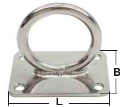
EYE PLATE WITH FIXED RING stamped AISI 304 ITEM NO. L mm B mm Ring mm B18-013 70 40 \Phi 8x45
