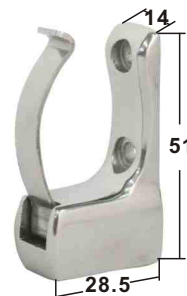
SPRING CLAMPS casted AISI 316 for boat hook ITEM NO. Min I.D. Weight/g 003116 1"(25mm) 42
