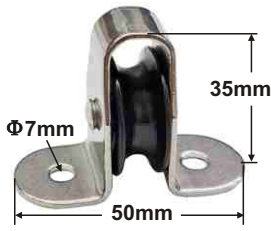
SINGLE LEAD BLOCK AISI 304 For rope \Phi 8mm plastic sheaves 30x11mm ITEM NO. Weight/g B23-049 31
