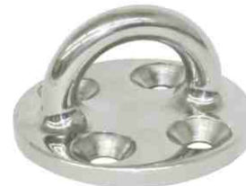
HEAVY DUTY ROUND PAD EYES AISI 316 ITEM NO. Base Dia Inside Dia Ring Dia Weight/g 003693 58mm (2-1/4") 17mm (11/16") 9.5mm (3/8") 6000kg(13200Lb)
