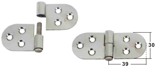
LIFT OFF HINGE stamped AISI 304 ITEM NO. Thickness Weight 008516 2.0mm 40g
