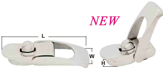
SNAP SHACKLE WITH SCREW AISI 316 (A4) ITEM NO. Thread L mm W mm Weight/g 004213 M6 40 35 40 004214 M8 52 46 90 004215 M10 72 57 270
