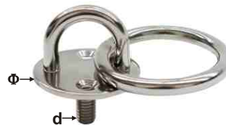
ROUND EYE PLATE WITH THREAD AND RING AISI 304 ITEM NO. \Phi mm Thickness d mm Ring Weight/g B19-024 33 2.5mm M6 5x30 40 B19-025 40 2.5mm M8 6x35 70 B19-026 50 3.0mm M10 8x45 140
